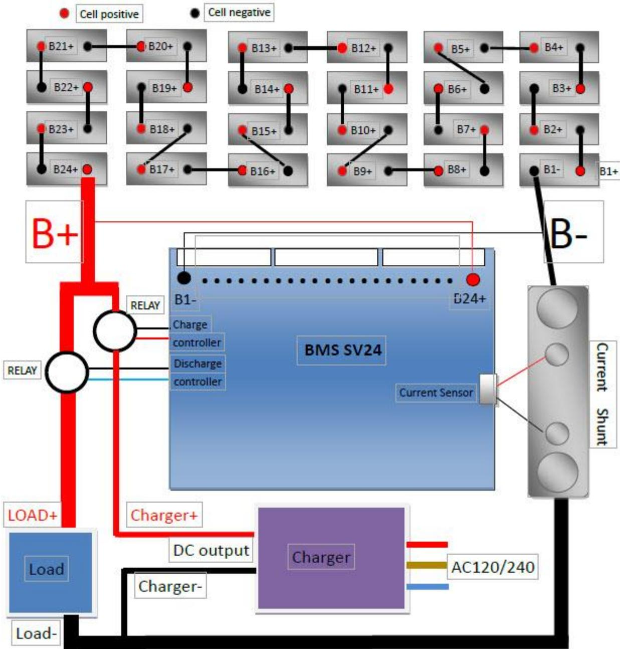
Heavy RED wires are positive of battery pack (B+/B24+), charger and load such as motor, and heavy black wire is negative of battery pack(B-/B1-), charger and load.
