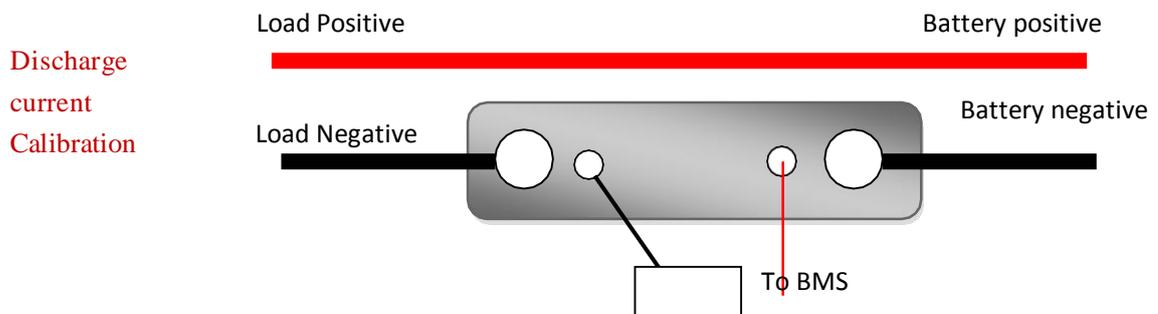
5. Press **SET/START** again and decrease the calibration current to new value (up to -125A, it must be less than current shunt, it is better to make it equal to your motor current, the key is the current must be accurate) turn on motor and discharge battery at the current, 3 seconds later, press **SET/START/** save the discharge calibration.
