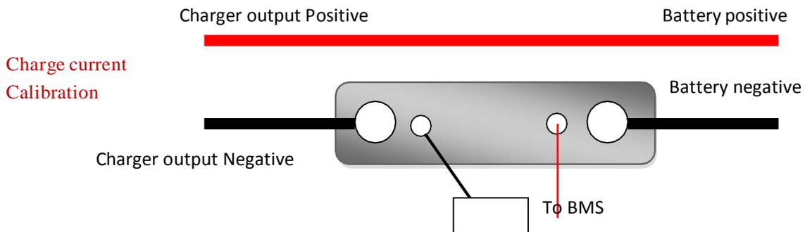
3. Shortly press **SET/START** make the current blink and increase the current to new value (up to 125A, it must be less than current shunt, it is better to make it equal to your charge current, the key is the current must be accurate), turn on charger and charge battery at the current, 3 seconds later, press **SET/START** save the charge current calibration.
