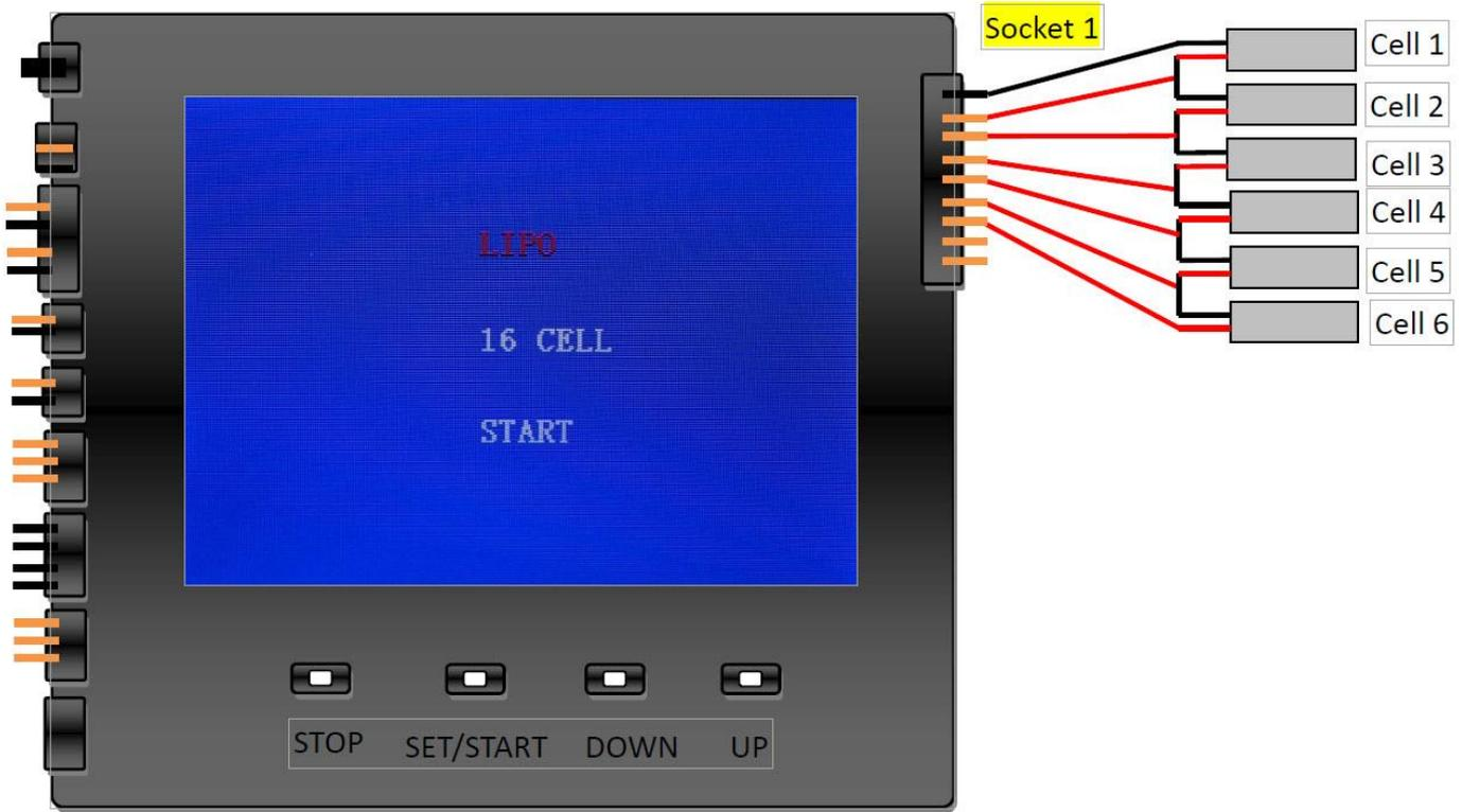
2. For over 8S battery pack, connect 8S to socket 1 and then socket 2 separately. Take 12S battery sample as following:
