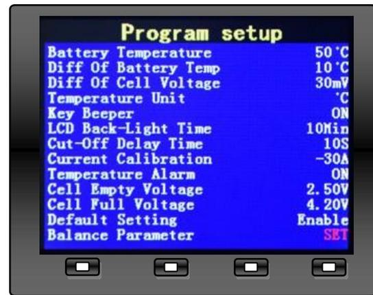
1. Press **SET/START** button for 3 seconds enter into Program Setup interface.
